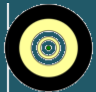
5mm round cable (TPU、LSZH、PE)
